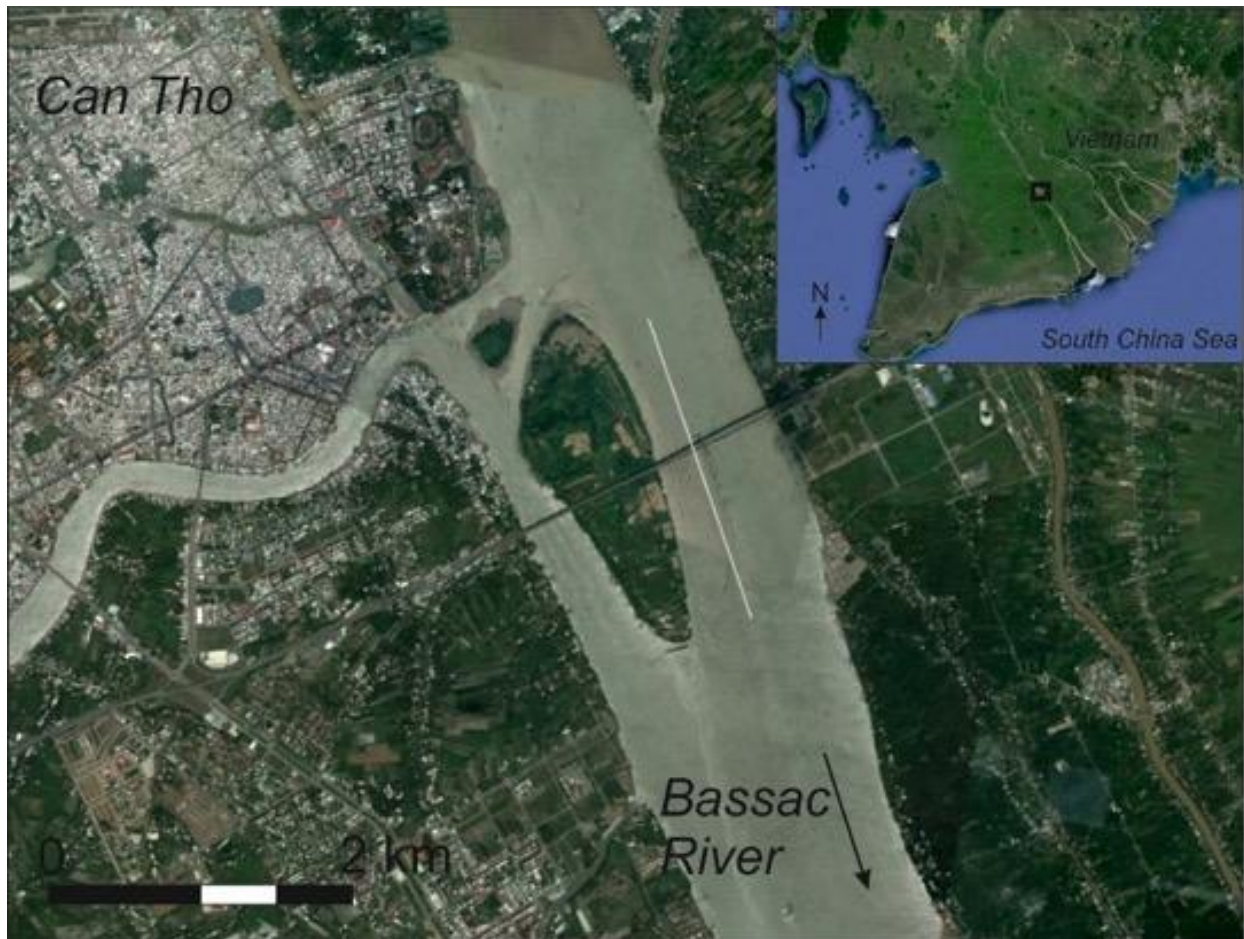
Figure 2: Map of the Mekong Delta and the study area: The white line indicates the track on the Bassac river, a distributary of the Mekong near the city of Can Tho, where the carbon dioxide and methane outgassing was monitored using the GasScouter (see Figure 3 for data). The efflux, flow dynamics and bed depth were monitored while drifting downstream.
