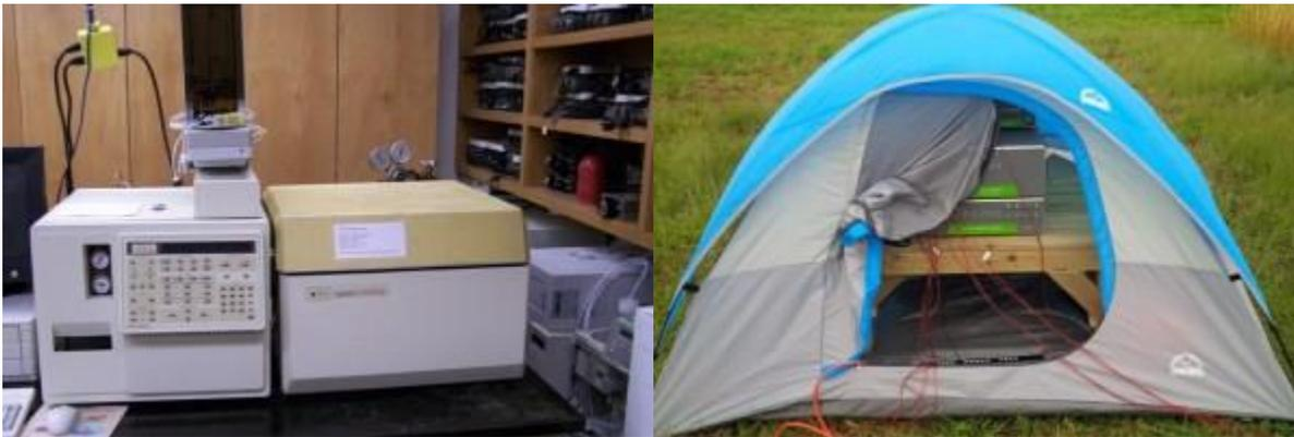
**Analysis of soil gas samples can be done using different methods: gas chromatography (GC, left) or laser-based spectroscopy (ie: [Picarro CRDS gas analyzer](#), right).**
