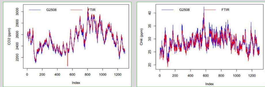
There was **good correlation** between the G2508 and the FTIR measurements of CO<sub>2</sub> and CH<sub>4</sub> from both the Pig and Dairy barns. Small differences between instruments lead to minor under- or over-estimation of absolute concentrations. Further inter-comparison is needed to evaluate measurements of N<sub>2</sub>O.
