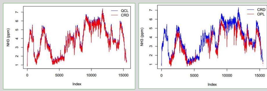
The G2508 showed **good accuracy** and **no evident drift over the two-month field tests**. Within all the tests in the dairy barn and the pig barn, the measured NH<sub>3</sub> concentration by G2508 was closer to the mean value of all methods. Boreal OPL and Emerson QCL were used for comparison.
