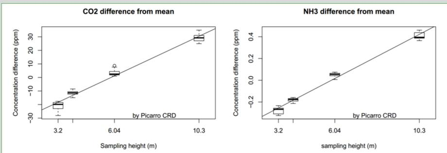
A **significant vertical variation** of gas distribution in the dairy barn was observed. Both NH<sub>3</sub> and CO<sub>2</sub> concentration increased with height. Little or no cross-ventilation lead to buoyancy dominating the vertical distribution of gases. **Horizontal variation was irregular** and the difference between test locations was not evident.
